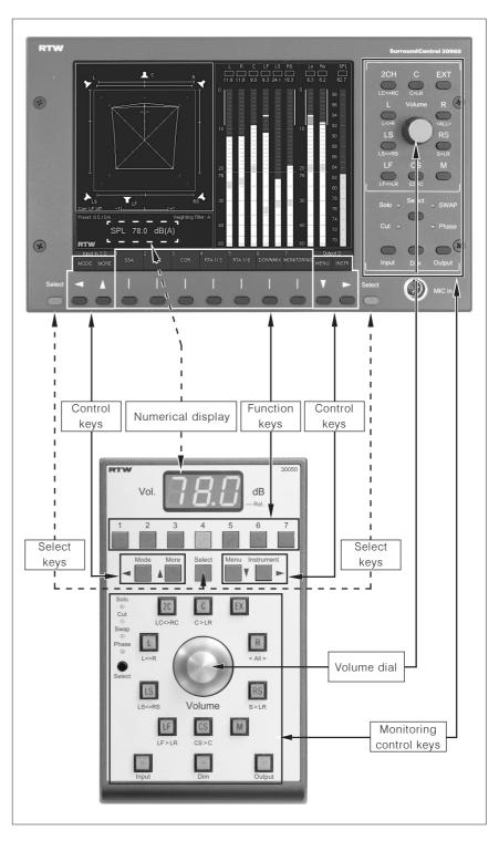
Fig. 4-2: The corresponding controls of the 31960 series
