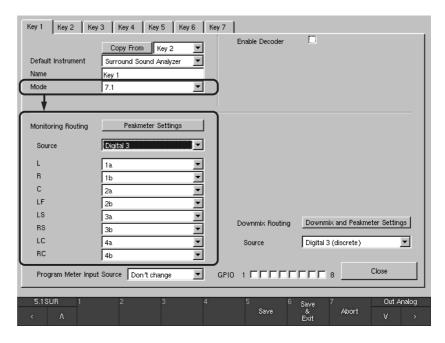
Fig. 6-29: The Monitoring Routing section in 7.1 Surround mode as an example
