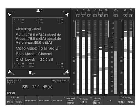
Fig. 2-10: The Monitoring controller instruments (MONITORING) displayed in window 3 (highlighted with a white frame)
