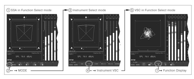
Fig. 5-3: Changing between Function Select and Instrument Select mode when selecting another instrument. Example with the instruments SSA and VSC
