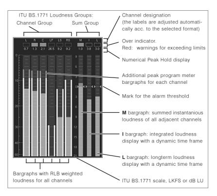
Fig. 5-8: Display elements of the Program Meter instrument in ITU BS.1771 Loudness mode with 5.1 surround format selected
