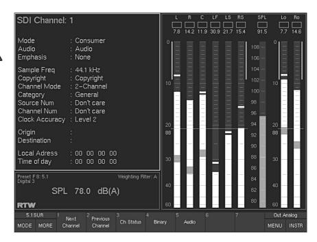
Fig. 2-13: The SDI status monitor instrument (SDI STATUS) displayed in window 3 (highlighted with a white frame)
