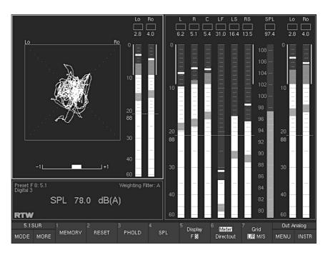
Fig. 5-29: The screen display with DOWNMIX instrument selected
