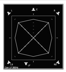
2. Identical sine wave signal with same level in the channels L, R, LS, RS. The correlation is  $r=\pm 1$  (outward broken TVI lines), the phantom sound sources (PSI) are in the middle, similar to a mono signal.
