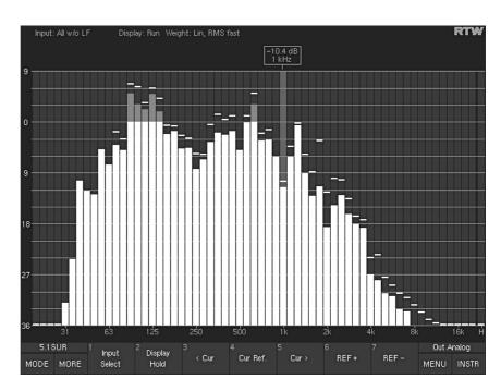
Fig. 2-8: The 1/6th octave Real Time Analyzer instrument (RTA 1/6) displayed in windows 2, 3, and 4
