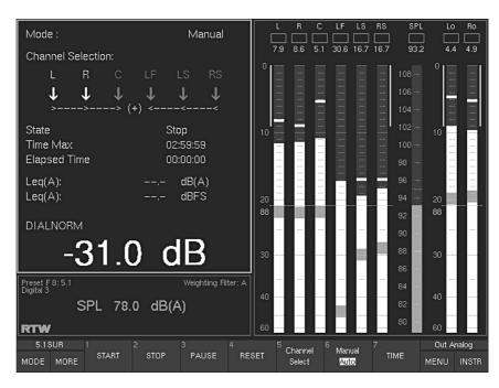
Fig. 5-57: The functions of the DIALNORM instrument displayed in the Toolbar
