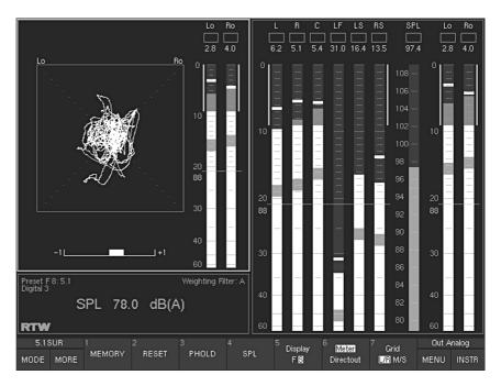
Fig. 2-9: The Two Channel Downmix Meter instrument (DOWNMIX) displayed in window 3 (highlighted with a white frame)
