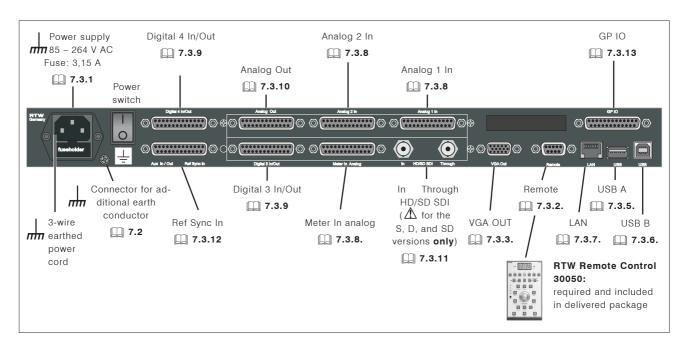
Fig. 7-1: Connectors on the rear panel of the SurroundControl 31900 series
