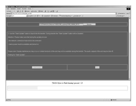
Fig. 8-9: Progress of the data transfer of the selected update file
