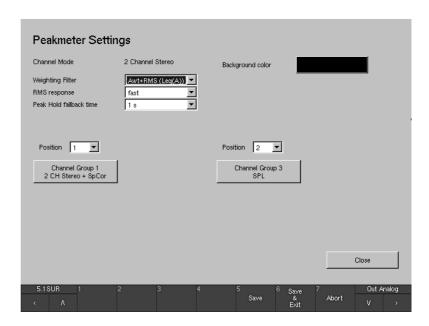
Fig. 6-37: The Peakmeter Settings menu page in 2 Channel Stereo mode
