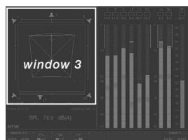
The VSC instrument is always displayed in window 3. To set the focus on this instrument (indicated by a highlighted frame around the window), simply press the **INSTR** key. With the focus on window 3, the VSC functions are displayed in the Toolbar (window 1).
