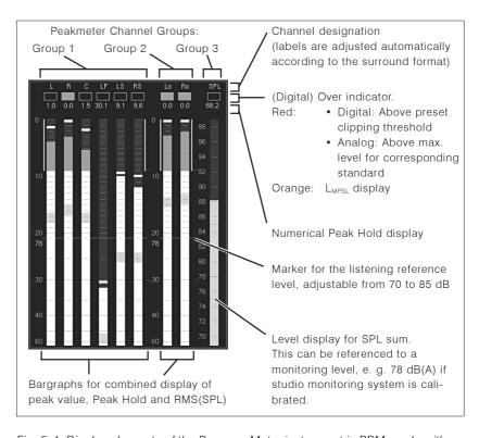
Fig. 5-4: Display elements of the Program Meter instrument in PPM mode with 5.1 surround format selected
