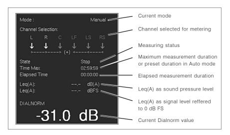
Fig. 5-56: The Dialnorm meter instrument (DIALNORM)
