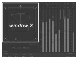
The DOLBY® META DATA instrument is always displayed in window 3. To set the focus on this instrument (indicated by a highlighted frame around the window), simply press the **INSTR** key. With the focus on window 3, the DOLBY® META DATA functions are displayed in the Toolbar (window 1).
