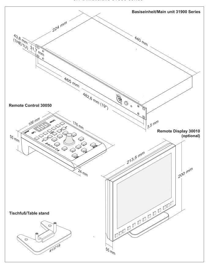
Fig. 9-1: Dimensions of the SurroundControl 31900 series system
