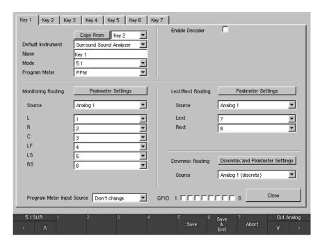
Fig. 6-20: Global Monitoring Input Routing menu page with "5.1" mode selected
