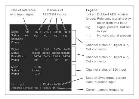
The HARDWARE STATUS instrument is always displayed in window 3. To set the focus on this instrument (indicated by a highlighted frame around the window), simply press the INSTR key. With the focus on window 3, the
