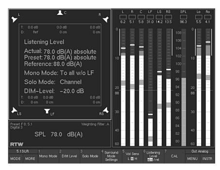
Fig. 5-31: First Toolbar function layer of the MONITORING instrument. Select MORE to display additional functions (layer 2)
