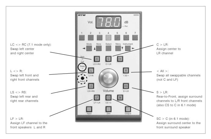
Fig. 4-4: Remote Control 30050 key assignments in Swap mode (31900 series) the same functions are available on the 31960 series control panel
