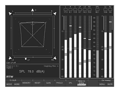
Fig. 2-2: Display elements of the Program Meter instrument in Window 2 (high-lighted with a white frame) with PPM mode in 5.1 Surround format selected
