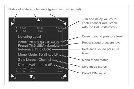
Fig. 5-30: The Monitoring Instrument (MONITORING)
