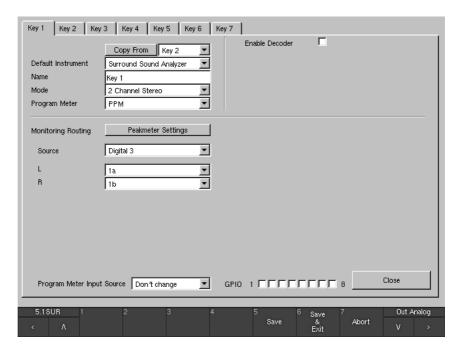
Fig. 6-18: Global Monitoring Input Routing menu page with "2 Channel Stereo" mode selected
