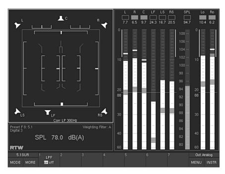
Fig. 2-6: The Correlator instrument (CORR) with phase meters for every channel pair displayed in window 3 (highlighted with a white frame)
