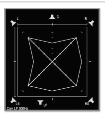
3. Same as on the left but with the phase of the left channel rotated through 180°. In the channel pairs L - R and L - LS each the correlation is r=-1, there are no phantom sound sources locatable.
