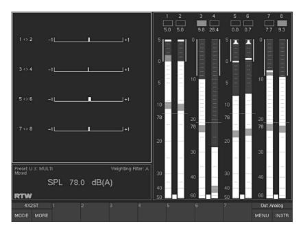
Fig. 5-20: The screen display with CORR instrument in Multi-Channel mode selected
