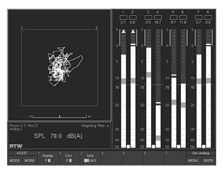
Fig. 5-16: The Audio Vectorscope instrument (VSC) in Multi-Channel mode
