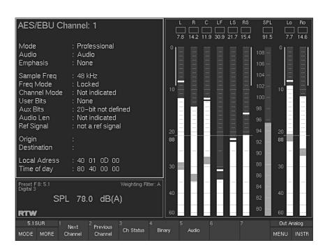
Fig. 2-12: The AES/EBU status monitor instrument (AES/EBU STATUS) displayed in window 3 (highlighted with a white frame)
