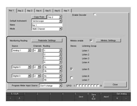
Fig. 6-31: The channels of the Multi-Channel mode devided in groups
