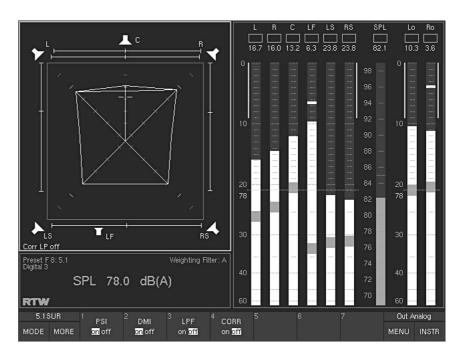
Fig. 5-12: The Surround Sound Analyzer (SSA) instrument in 5.1 surround mode
