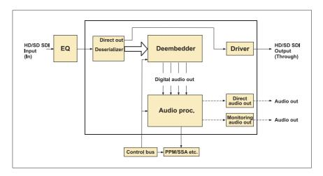
Fig. 7-5: Block diagram of the HD/SD SDI interface
