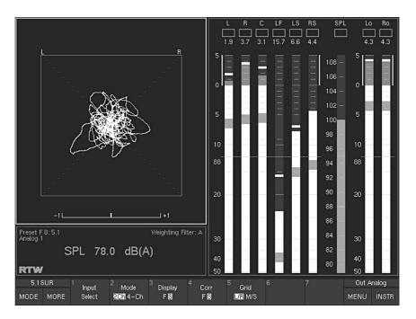
Fig. 2-5: The Audio Vectorscope instrument (VSC) displayed in window 3 (high-lighted with a white frame)
