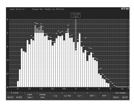
Fig. 5-22: First Toolbar function layer of the RTA instruments in 5.1 Surround mode. Select MORE to display additional functions (level 2) (Example: RTA 1/6)
