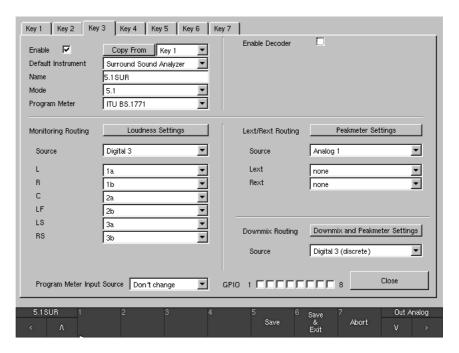
Fig. 3-16: The Key 1 to 7 Sub Preset menu tabs of the Monitoring Input Routing setting with ITU BS.1771 selected for Program Meter
