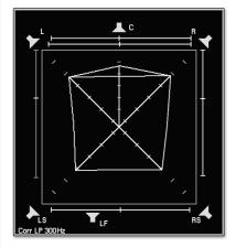
4. Surround signal with some Center presence (roof). A support microphone would be too dominant. A dialog in relation to music would be too quiet. The width of the PSI lines of the C channel is a sign of coherent signal parts in L and/or R (crosstalk).
