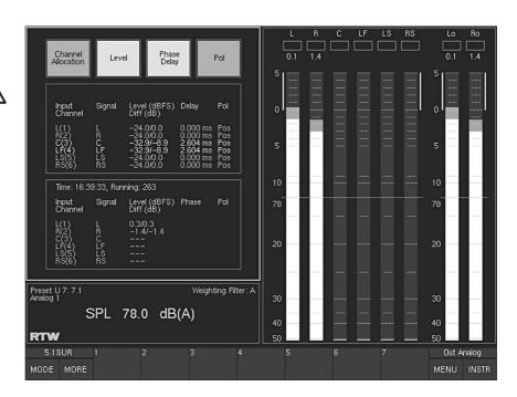
Fig. 2-18: The Dialnorm Meter instrument (DIALNORM) displayed in window 3 (highlighted with a white frame)
