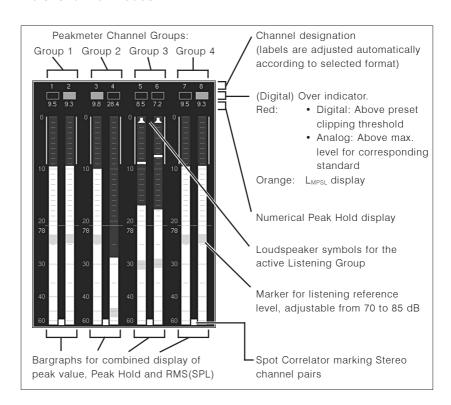
Fig. 5-5: Display elements of the Program Meter instrument in PPM mode with Multi-Channel format selected
