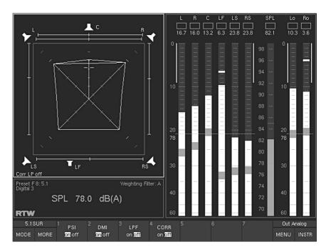
Fig. 2-4: The Surround Sound Analyzer instrument (SSA) displayed in Window 3 (highlighted with a white frame)
