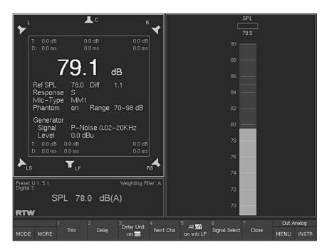
Fig. 5-33: First Toolbar function layer of the CAL instrument. Select MORE to display additional functions (layer 2)
