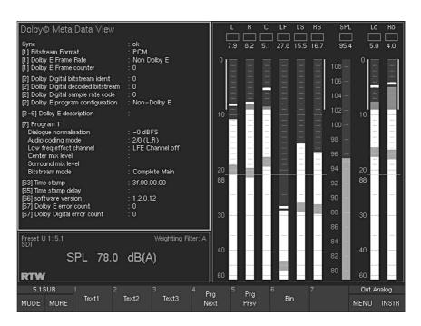
Fig. 5-51: The functions of the DOLBY® META DATA instrument displayed in the Toolbar
