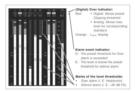
Fig. 6-57: Display elements of the Program Meter instruments alarm functions. Example: PPM in 5.1 surround mode
