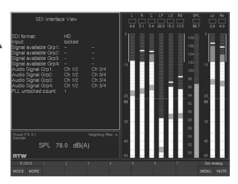
Fig. 2-14: The SDI interface monitor instrument (SDI INTERFACE) displayed in window 3 (highlighted with a white frame)
