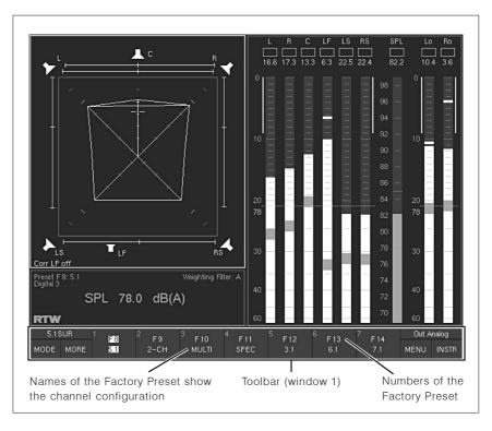
Fig. 3-4: Factory Presets displayed in the Toolbar (window 1)
