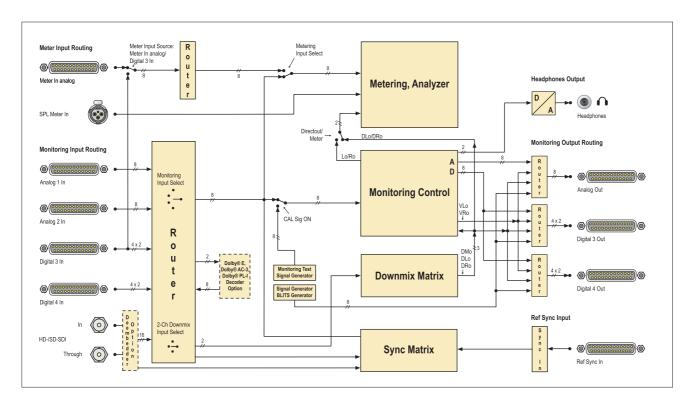
Fig. 6-6: Signal routing in the SurroundControl units
