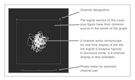
Fig. 5-14: The Audio Vectorscope instrument (VSC)
