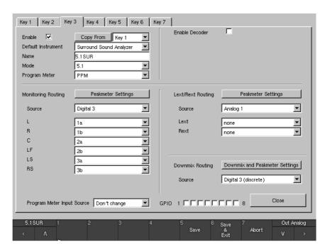
Fig. 3-12: The Key 1 to 7 Sub Preset menu tabs of the Monitoring Input Routing setting
