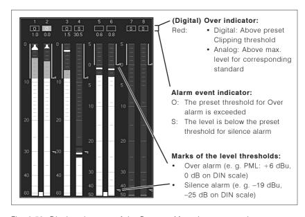
Fig. 6-58: Display elements of the Program Meter instruments alarm functions. Example: PPM in Multi-Channel mode
