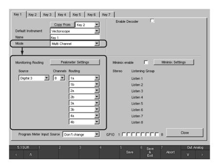
Fig. 6-30: The Monitoring Routing section with Multi-Channel mode selected
