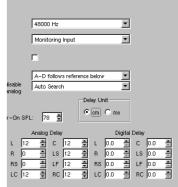
Fig. 6-51: Comparison of the entered negative delay values in the CAL instrument and the displayed values on the Audio System menu page
