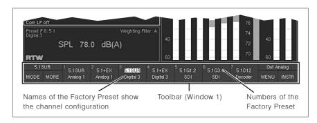
Fig. 6-5: Sub Presets 1 to 7 displayed in the Toolbar in Window 1
