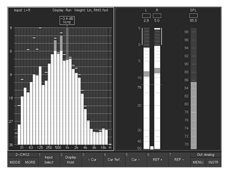
Fig. 5-26: First Toolbar function layer of the RTA instruments in 2-Channel Stereo mode. Select MORE to display additional functions (layer 2)
