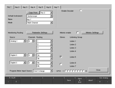
Fig. 6-24: Global Monitoring Input Routing menu page with "Multi Channel" mode selected (4-Channel, 2-Channel Stereo, 2-Channel)
