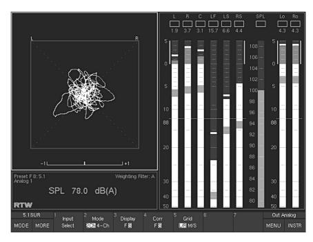
Fig. 5-15: The Audio Vectorscope instrument (VSC) in 5.1 Surround mode
