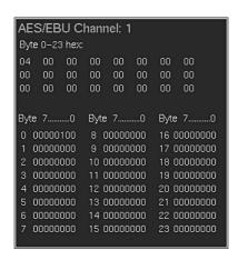
Fig. 5-43: Screen display of window 3 after selecting the Binary function
