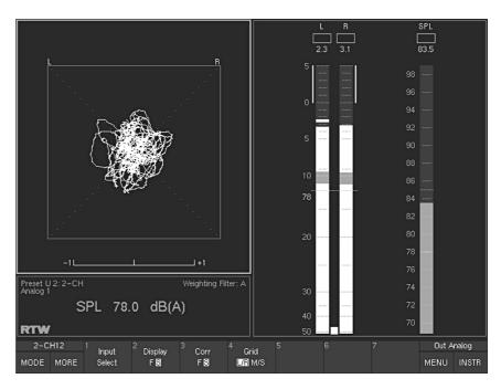
Fig. 5-17: The Audio Vectorscope instrument (VSC) in 2-Channel Stereo mode
