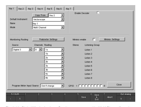
Fig. 6-23: Global Monitoring Input Routing menu page with "Multi Channel" mode selected (8-Channel)
