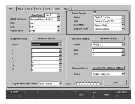
Fig. 6-28: Example for the enabled Dolby® decoder (only with D and SD versions)
