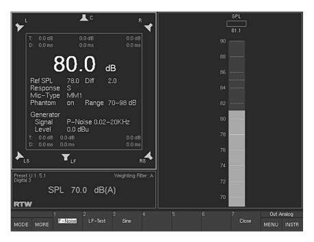
Fig. 5-35: Display after selecting the Signal Select function of the CAL instrument
