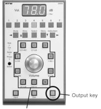
Channel keys and volume control on the Remote Control 30050 Also see Figs. 4-2 and 4-3
