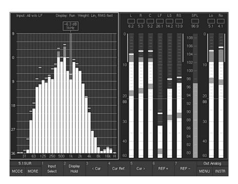
Fig. 2-7: The 1/3rd octave Real Time Analyzer instrument (RTA 1/3) displayed in window 3 and window 4 (highlighted with a white frame)
