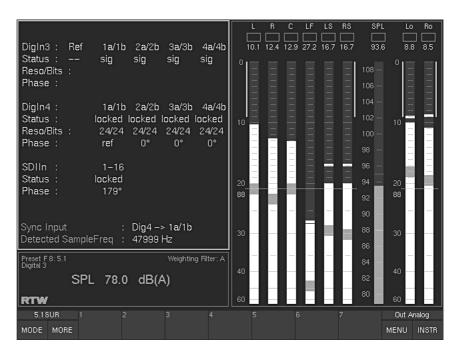
Fig. 2-15: The Hardware Status monitor instrument (HARDWARE STATUS) displayed in window 3 (highlighted with a white frame)
