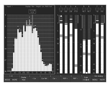
Fig. 5-24: First Toolbar function level of the RTA instruments in Multi-Channel mode. Select MORE to display additional functions (layer 2)
