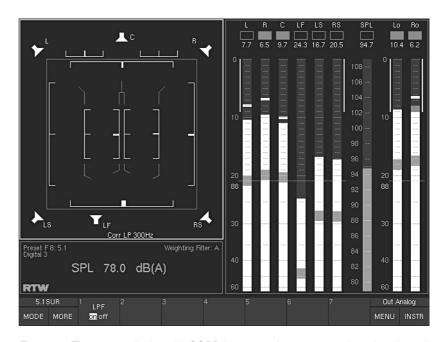
Fig. 5-19: The screen display with CORR instrument in 5.1 surround mode selected
