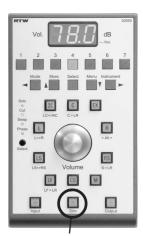
**DIM** key on the Remote Control 30050 **DIM** key also see Figs. 4-2 and 4-3 and Chapter 4.3.13
