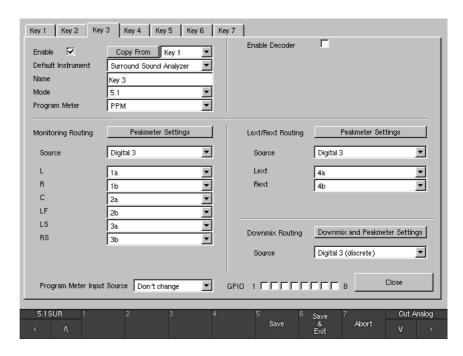
Fig. 6-17: The Key 1 to 7 menu tabs after pressing the Monitoring Input Routing button (screen content might change depending on the channel format used)
