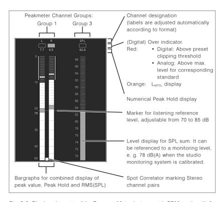
Fig. 5-6: Display elements of the Program Meter instrument in PPM mode with 2-Channel Stereo format selected
