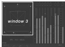
The DOWNMIX instrument is always displayed in window 3. To set the focus on this instrument (indicated by a highlighted frame around the window), simply press the **INSTR** key. With the focus on window 3, the DOWNMIX functions are displayed in the Toolbar (window 1).
