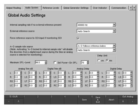
Fig. 3-2: The Audio System menu tab with the Global Audio Settings menu
