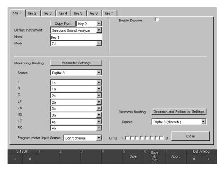
Fig. 6-22: Global Monitoring Input Routing menu page with "7.1" mode selected
