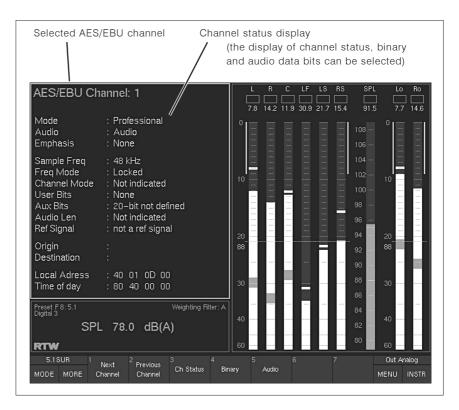
Fig. 5-42: The AES/EBU channel status monitor (AES/EBU STATUS)
