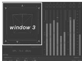
The SDI INTERFACE instrument is always displayed in window 3. To set the focus on this instrument (indicated by a highlighted frame around the window), simply press the **INSTR** key. With the focus on window 3, the SDI INTERFACE functions are displayed in the Toolbar (window 1).
