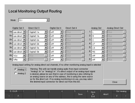
Fig. 3-13: The Local Monitoring Output Routing menu
