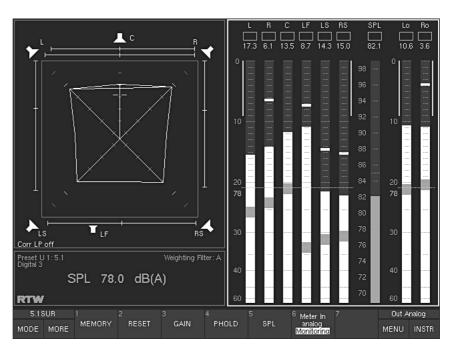
Fig. 5-7: The functions of the PPM instrument displayed in the Toolbar
