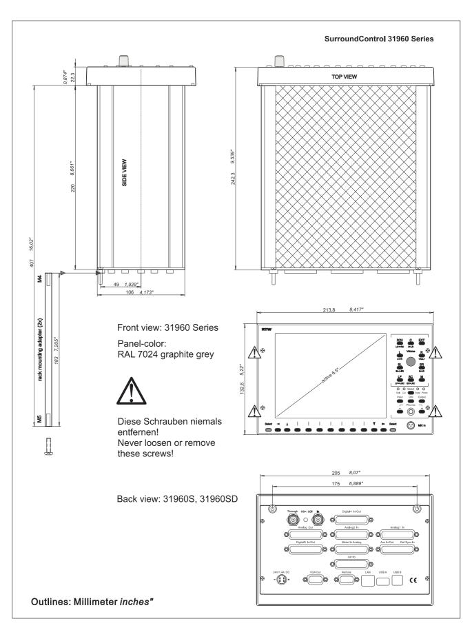
Fig. 9-1: Dimensions of the SurroundControl 31960 series
