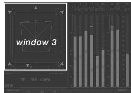
The AES/EBU STATUS instrument is always displayed in window 3. To set the focus on this instrument (indicated by a highlighted frame around the window), simply press the **INSTR** key. With the focus on window 3, the AES/EBU STATUS functions are displayed in the Toolbar (window 1).
