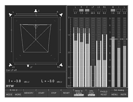
Fig. 2-3: Display elements of the Program Meter instrument in window 2 (highlighted with a white frame) with ITU BS.1771 Loudness Meter mode selected in 5.1 surround format, combined with peakmeter display
