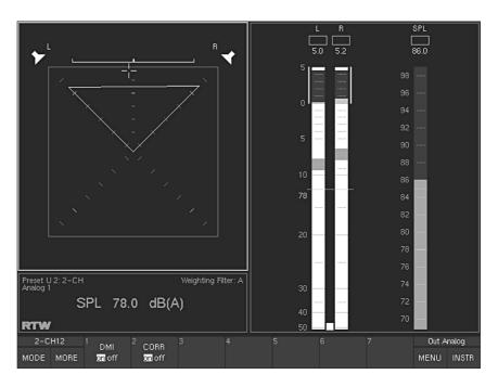
Fig. 5-13: The Stereo Sound Analyzer (SSA) instrument in 2-Channel Stereo mode
