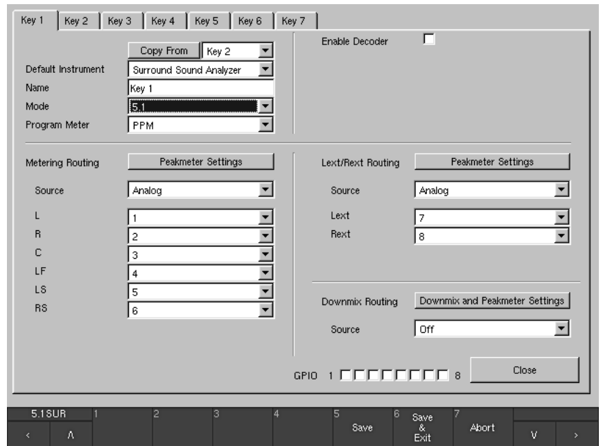
Fig. 6-19: Global Input Routing menu page with „5.1“ mode selected
