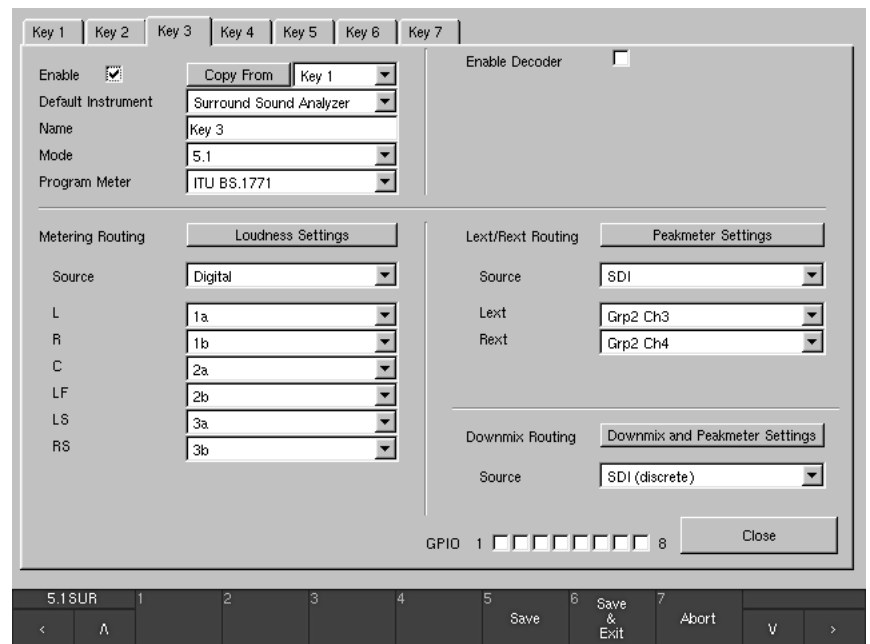
Fig. 3-15: The Key 1 to 7 Sub Preset menu tabs of the Input Routing setting with ITU BS.1771 selected for Program Meter
