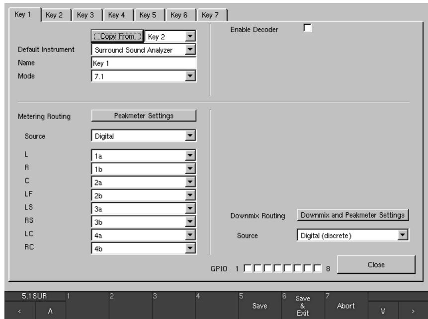
Fig. 6-21: Global Input Routing menu page with „7.1“ mode selected
