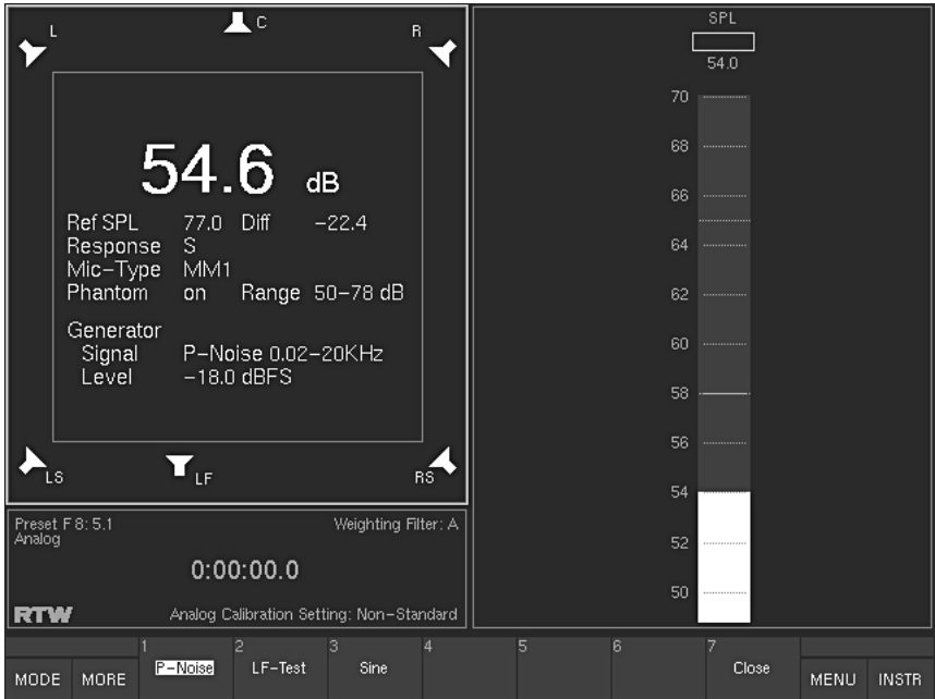
Fig. 5-28: Screen display after selecting the Signal Select function of the CAL instrument
