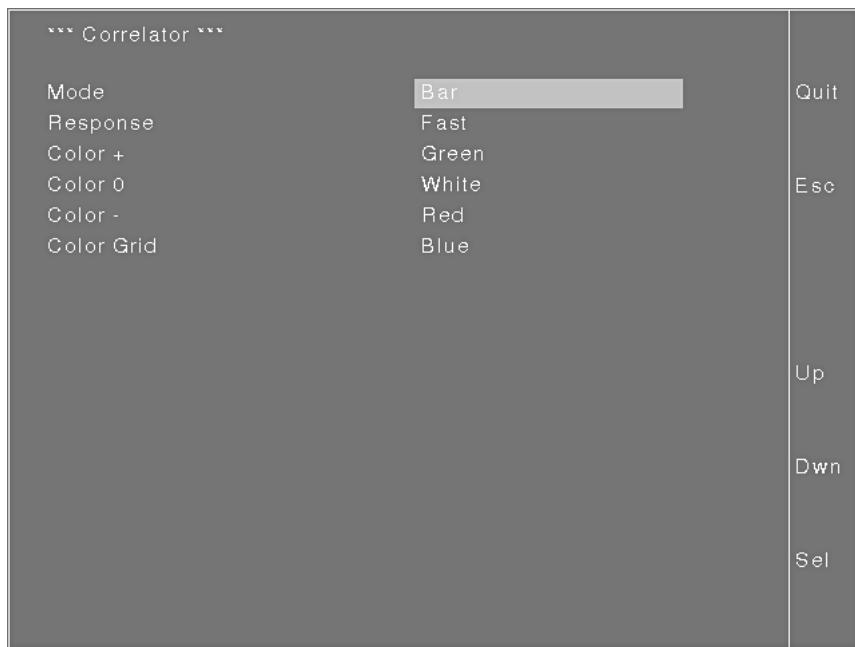
Fig. E 4-17: Correlator menu display with Correlator parameters
