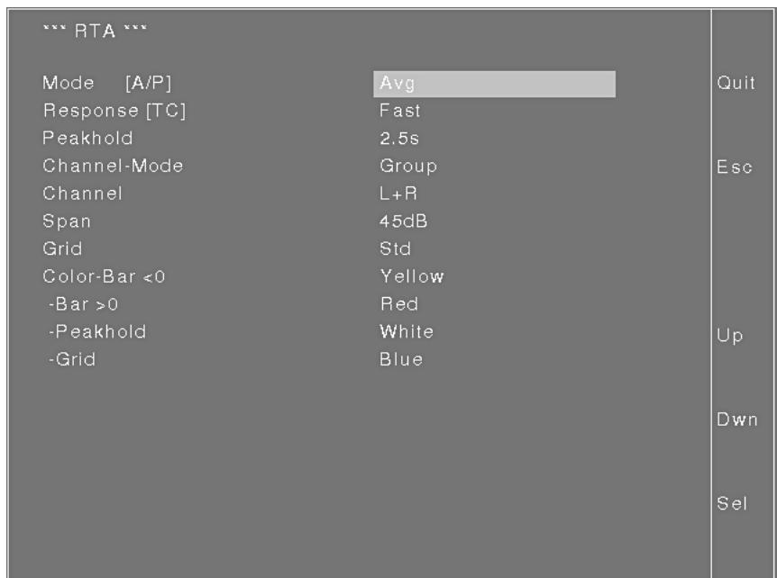
Fig. E 5-14: The more .. submenu for Primary Function: RTA
