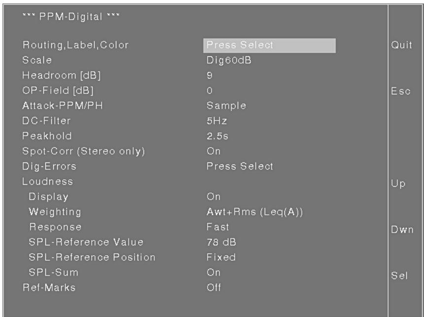
Fig. E 5-4: The PPM-Digital submenu
