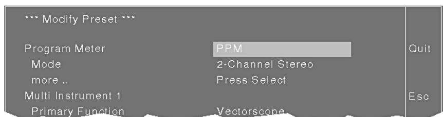
Fig. E 4-2: The Program Meter selection in PPM mode
