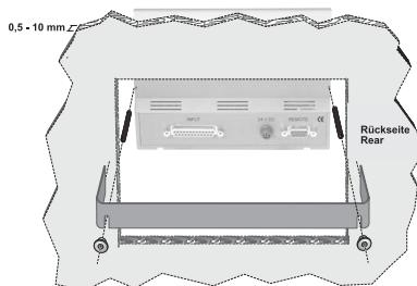
Panel mounting kit **13713** for front panel installation
